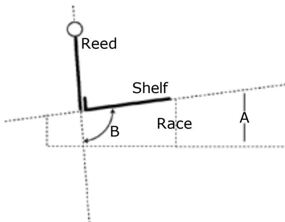
If the box shelves are lower or higher than the race, you'll need to loosen the bolts in the large Box Mounting Bracket that attaches the Shuttle Box Assembly to the side of the loom. This will allow you to make the necessary adjustment.
